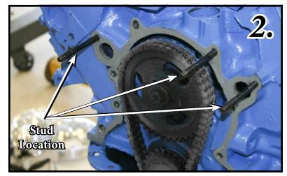
*Fig-3:* Apply a thin coat of RTV silcone sealant to a new timing cover gasket and oil pan to timing cover gaskets. Install timing cover and (P500) water pump to block. Secure using the Three Threaded Stainless Spacer (S769) as shown in *Fig-3*. Add water pump and timing cover bolts in locations D, E, and F, (See Fig 1 for proper placement and bolt sizes.) Do not forget to reinstall the four factory bolts through the oil pan and into timing cover.
