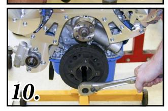
*Fig-11:* Apply Loc-Tite to the threads of the four (S186) <sup>5</sup>/<sub>16</sub> -24 x <sup>7</sup>/<sub>8</sub>" SHCS. Place the water pump pulley (2282-A) and (322-A)Water Pump Cap to the water pump and thread the cap screws through pulley and into water pump pulley flange, tighten firmly (28 ft/lbs.) Install (221) Alternator Fan, (S685) Lock Washer and (206-A) Alternator Pulley.
