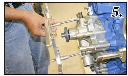
Fig-6: Install (P572) Alternator, Line up (30412-A) Rear Alternator support with front main bracket installation hole. Use a (S278) 3/8 x 5" SHCS, adjust Threaded Bushing (S450) to take up any slack between Alternator Lower Mount and brackets. Leave
