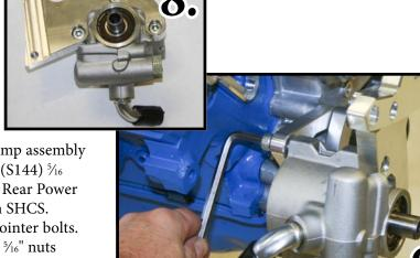
*Fig-9:* Install the power steering bracket and pump assembly to the Main Front Bracket (30411-A) with Two (S144)  $\frac{5}{16}$  -18 x  $\frac{7}{8}$ " SHCS. Also secure pump to (30414-B) Rear Power Steering Bracket using One (S550) M8 x 20 mm SHCS. Tighten all front and rear support and timing pointer bolts. For kits without Power steering use Two (S616)  $\frac{5}{16}$ " nuts along with the (S144)  $\frac{5}{16}$  -18 x  $\frac{7}{8}$ " SHCS to fill the holes.
