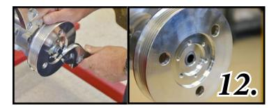
*Fig-13:* Install Dayco #5060595 59½" (#5060575 57½" without power steering) 6 Rib Belt by removing the top A/C Bolt and (MM100) bushing and allowing it to swing inward past the slot. Install belt as shown pull back A/C unit reinstall (MM100) bushings and M8 SHCS.
