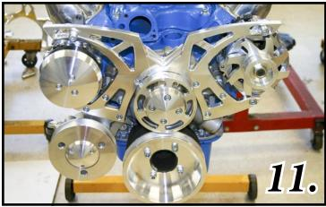
*Fig-12:* Press (618-A) Power Steering Pulley on with a install tool or bolt and washer as shown. When properly installed pulley should be flush with top of shaft as shown and aligned with crank pulley.
